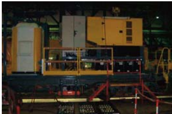
Electric motorisation of works train wagons
