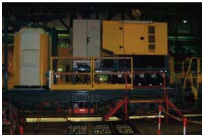
Electric motorisation of works train wagons
